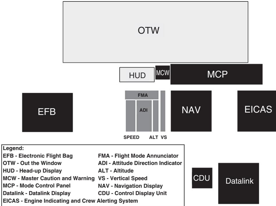
Figure 1. Instrument panel layout upon which model was exercised. The AOI [AQ: 6] corresponding to the to-be-noticed event is not shown here but was positioned as required for the particular model runs.
